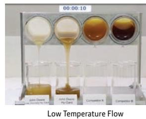
Hy-Gard and Low Viscosity Hy-Gard are checked for proper viscosities using the slow-cool fluidity test in addition to industry-standard tests. The slow-cool fluidity test (developed by John Deere engineers and recognised by the oil industry as a valid testing procedure) ensures Hy-Gard's proper viscosity performance, which reduces downtime and lowers the cost of operation. Few competitive hydraulic transmission oils are tested for this type of low-temperature viscosity performance.
