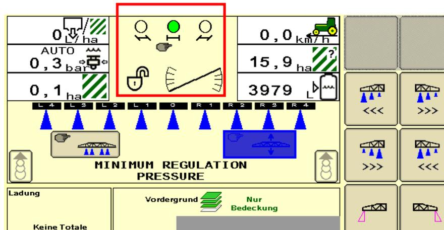
When lock and/or drawbar steering is not equipped, the lock status and drawbar status is not visible.
