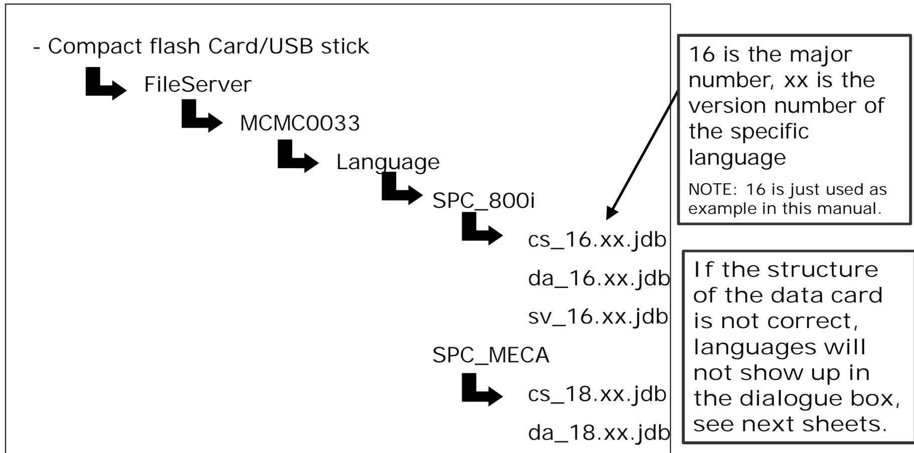
CF-card can have more sub-directories (like RCD), depending on the use. When downloaded via Stellar Support, the structure will be created automatically.
