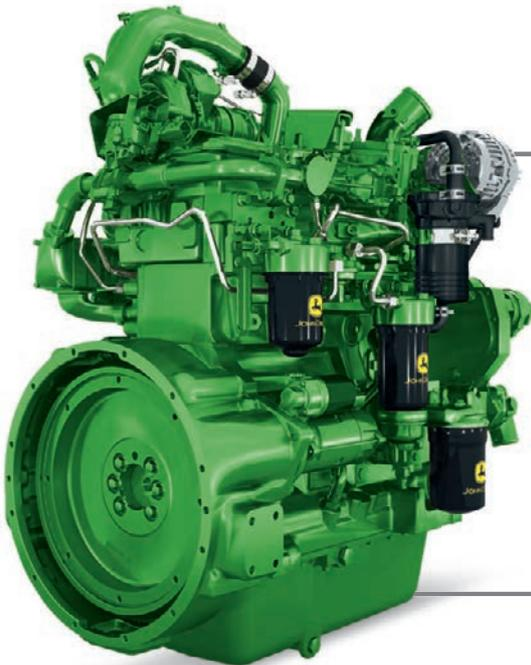
Our 4.5 L PSS engines (6R 110, 6R 120, 6R 130, 6R 140 and 6R 150) use a 2-stage turbocharging system in which the Wastegate turbocharger multiplies the pressure created by a fixed vane turbocharger. This sequential arrangement boosts power to achieve up to 131 kW (177 hp, max with IPM) in the 6R 150.
