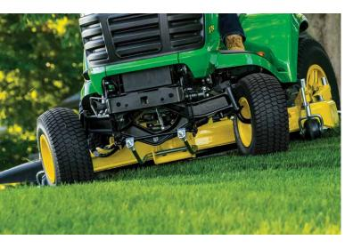
No scuffing. The speed of each front wheel adjusts automatically on turns in our full-time 4-wheel-drive system.
