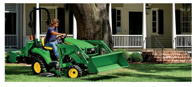
Never alter the roll over protective structure (ROPS) unless approved by the manufacturer. Damaged ROPS must be replaced, not repaired or serviced.
