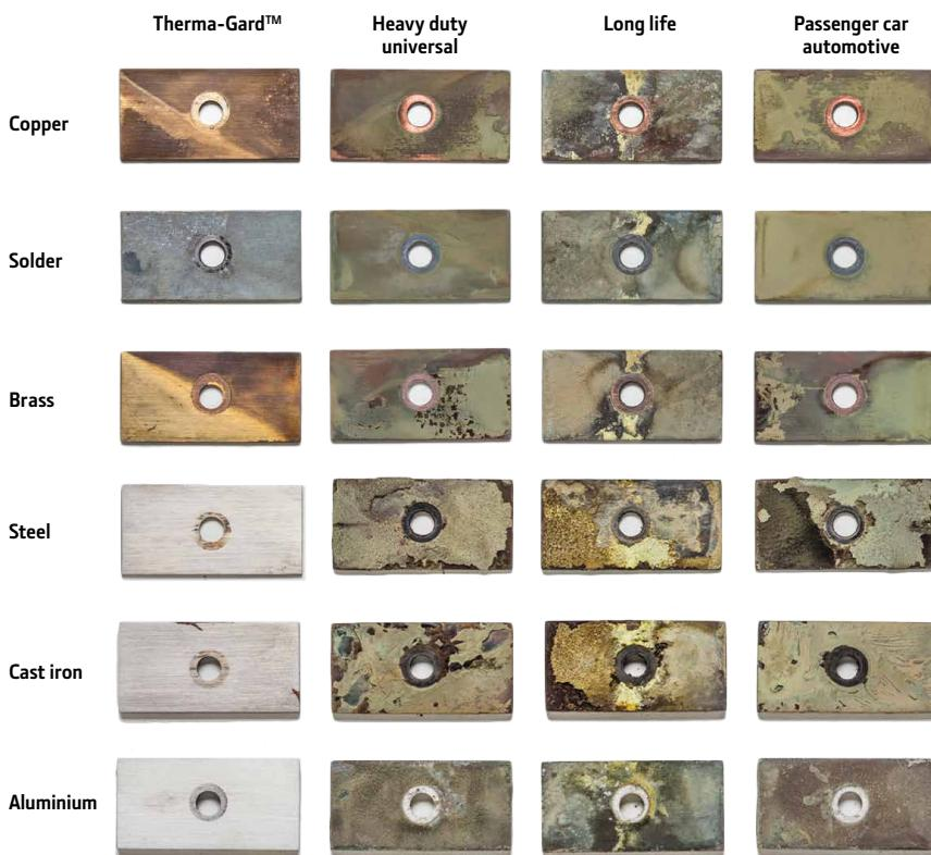
Therma-Gard extends the life of your water pump. Moving components in the cooling system, such as water pump impellers are also subject to cavitation problems. Incorrect coolant promotes erosion of the water pump impeller and the surrounding areas. You can prevent this type of problem by using Therma-Gard.
