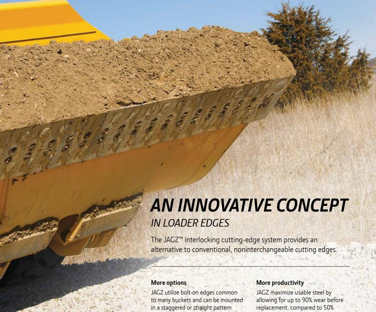
to many buckets and can be mounted in a staggered or straight pattern depending on your application. When mounted in a staggered pattern, you get increased penetration and better bucket fill. The straight pattern leaves a smoother working surface, making it perfect for loading. JAGZ also balance wear by swapping the more quickly worn outside edge with the less worn centers.
