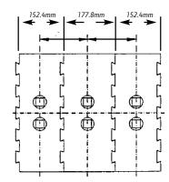
A 7-IN. JOINER WITH 6-IN. SEGMENTS AT BOTH SIDES
