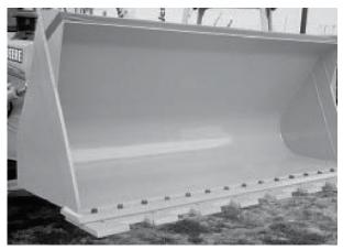
Backhoe loader bucket equipped with T825330 (25.4mm x 152.4mm x 301.63 mm, <sup>5</sup>/<sub>8</sub>-in. bolts) short standard sections, and T825333 and T825334 end sections.
