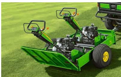
**22B utility trailer**: The multi-angle ramp makes it easy to transport walk behind mowers to the next green.
