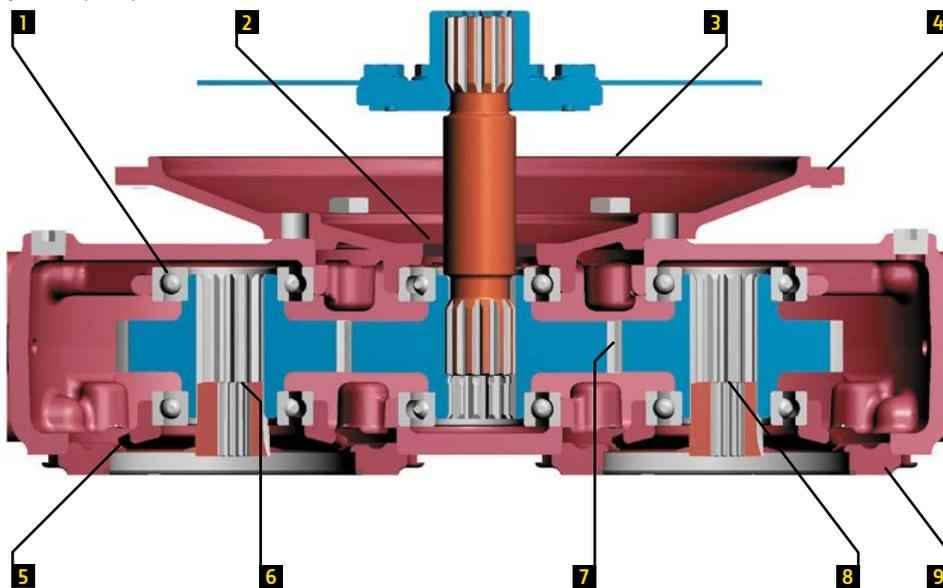
**1 Ball bearings** include a built-in oil reservoir in the outer race to provide uninterrupted lubrication.
