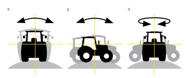
Reliable everywhere — The Terrain Compensation Module (TCM) detects and assesses roll (x), pitch (y) and yaw (z) to ensure true machine ground positioning across every field.
